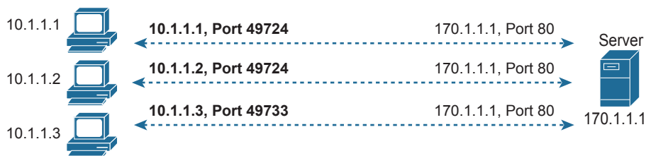
Figure 10-6 Three TCP Connections from Three PCs
