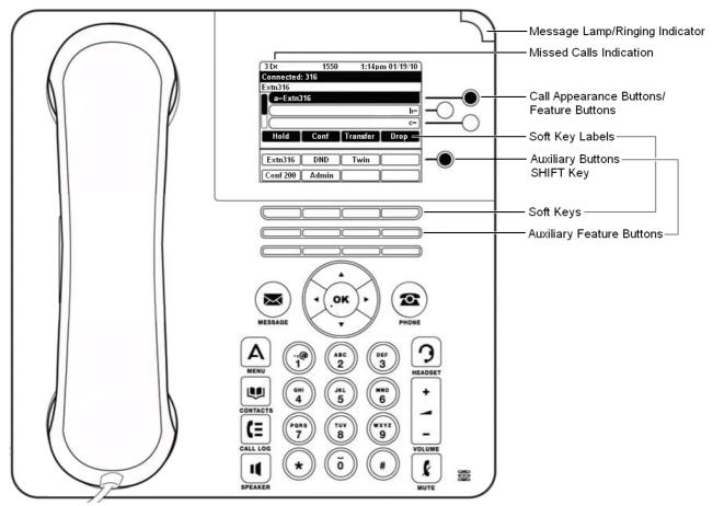
The phone supports 24 programmable call appearance/feature buttons. The labels for 3 of these are displayed in the main display and can be controlled by the adjacent buttons to the right. You can use the  $\blacktriangle$  up and down  $\P$  arrow keys to scroll the display. You can also use the  $\blacktriangleleft$  left and right  $\blacktriangleright$  arrow keys to move through the button feature in pages of 3.
