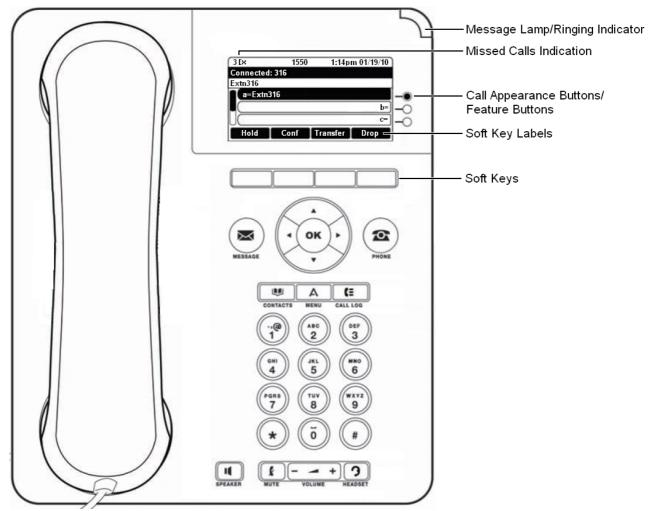
The phone supports 12 programmable call appearance/feature buttons. The labels for 3 of these are displayed in the main display and can be controlled by the adjacent buttons to the right. You can use the  $\blacktriangle$  up and down  $\P$  arrow keys to scroll the display. You can also use the  $\blacktriangleleft$  left and right  $\blacktriangleright$  arrow keys to move through the button feature in pages of 3.
