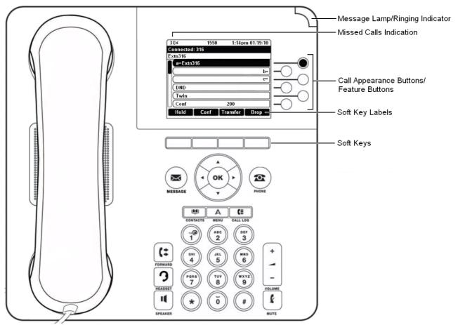
The phone supports 24 programmable call appearance/feature buttons. The labels for 6 of these are displayed in the main display and can be controlled by the adjacent buttons to the right. You can use the  $\blacktriangle$  up and down  $\forall$  arrow keys to scroll the display. You can also use the  $\blacktriangleleft$  left and right  $\blacktriangleright$  arrow keys to move through the button feature in pages of 6.
