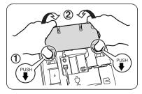
KX-T7730 model illustrated on this page. 3 Mount the unit on the wall.
