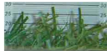
Figure 2 – example of Free pile height measurement
