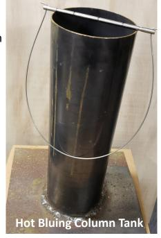
Once the salts are heated, the actual bluing process takes a little over a half hour for a set of three knives, including two plunges into ice water (deepens the blue/black). Of course, it's not scratch resistant (What finish is?) and care must be taken to keep dry when not in use, but if you're just sticking wood, the finish will last a very long time. Any questions?
