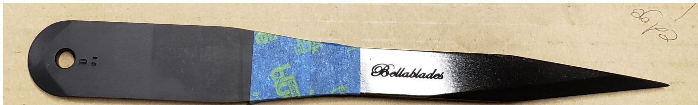
Painted blade after laser etch.
