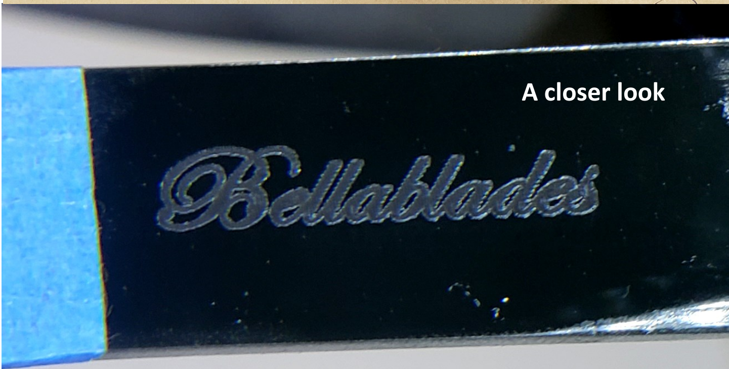
Painted blade after laser etch.
