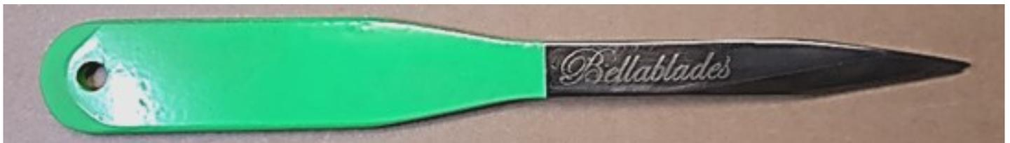
8. By the third refurb the powder coat was almost gone. Constant knife-on-knife action stripped away most of it over a period of ~ 7 months. Worst loss from original length ~ 0.120", mostly from reshaping tip and rear bevel, not chipping. Loss of weight from original < 3 grams. No perceptible change in balance point.
