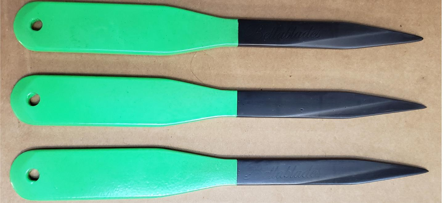
6. Speaking of abuse, this one is the result of the first refurb. Refurbs are for inspection and restoring the Neon Green Powder coat! The first refurb was done ~ 4 months after making them.
