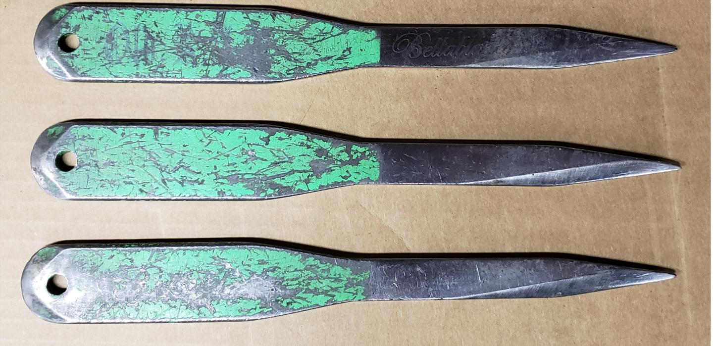
2. After a bit of belt sanding with 120 grit to strip remaining powder coat and smoothen edges (mostly rear bevel due to multiple direct and deflected hits), I buffed with 150 grit loaded on a wheel.
