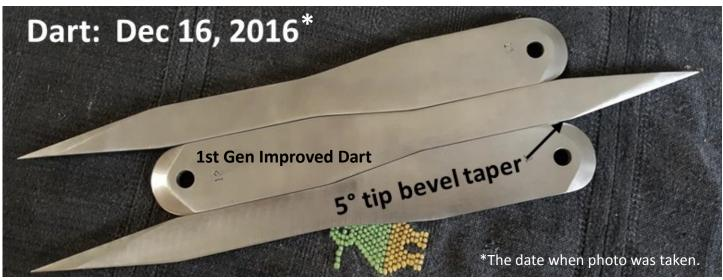
The reason for calling them "Improved" was the rear bevel. It did fit the hand nicely, but its main function was to reduce the probability of an impact on the back of the handle from another knife. The one above was the first attempt at improvement. The primary variable over time has been the tip bevel taper. The 5° tip taper was also used on <u>all</u> of our previous knives, as well.
