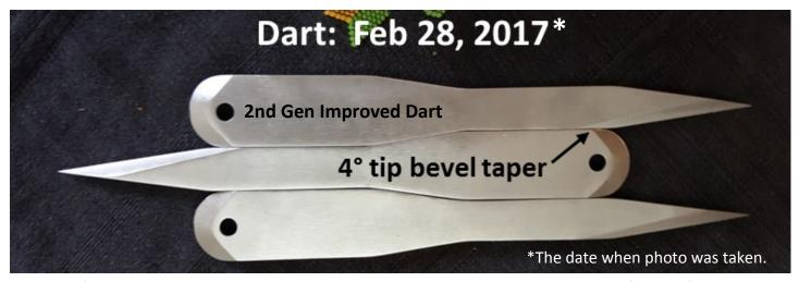
In order to further improve penetration, we tried a 4° tip bevel taper, shown above. We made several of these before testing a 3° tip bevel taper. We still prefer 4° for our thicker knives. These were also the first knives to be heat treated in our electric furnace.
