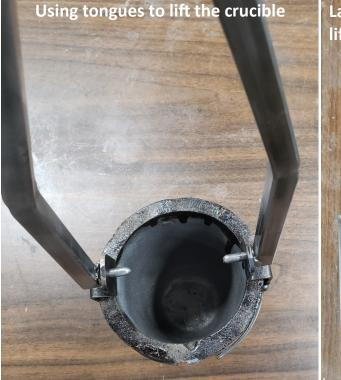
Large crucible with lift ring, tongues attached to lift ring, larger pouring ring
