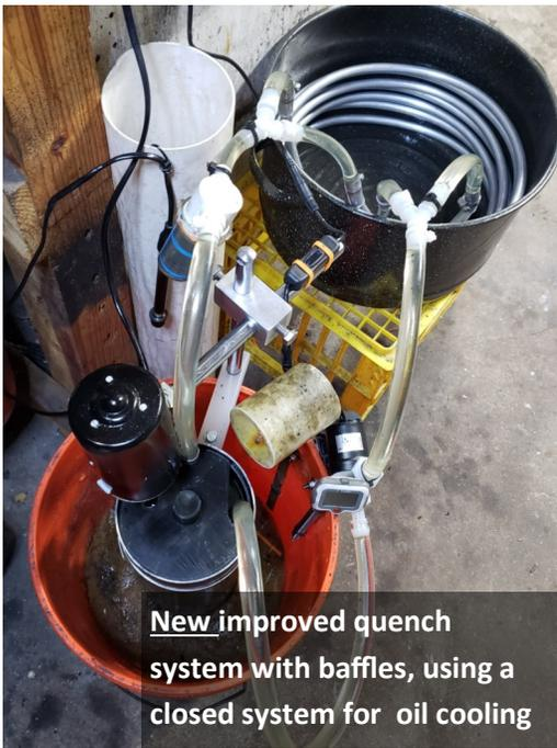
New improved quench system with baffles, using a closed system for oil cooling
