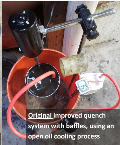
Original improved quench system with baffles, using an open oil cooling process
