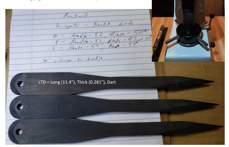
As you can see below, I hit my stated hardness targets of HRC 50  $\pm$  1, with the exceptions of LTD 4 handle and LTD 5 blade. I believe the HRC 47 was an inaccuracy caused by a minor bend that was only noticeable when sliding a piece of paper under the other side of that Dart. Also I recorded values within  $\pm$  0.5 units. Looking at the Rockwell increments of the gauge, there is no reason to attempt to be more accurate.
