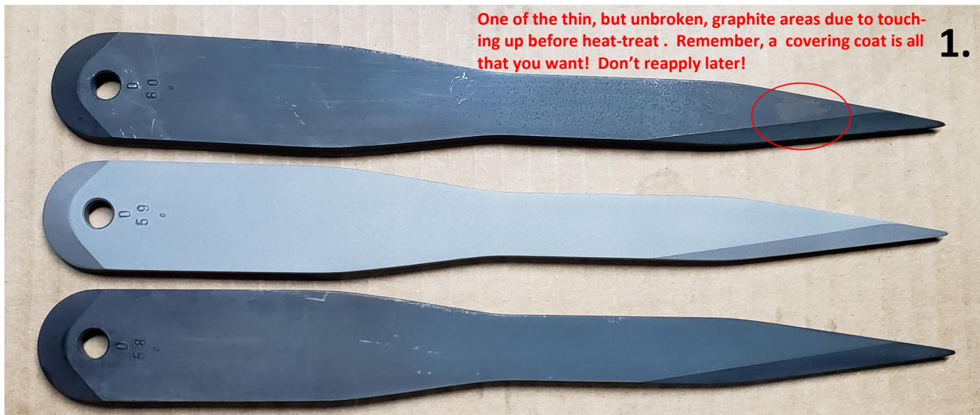
1. D59G after 80 grit garnet blasting, compared to before (D58G and D60G after heat-treating).
