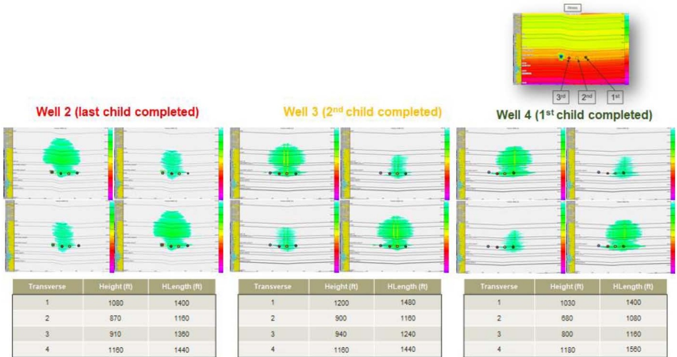
Figure 14—Completions – In-fill child well fracture pressure history matching hydraulic lengths
