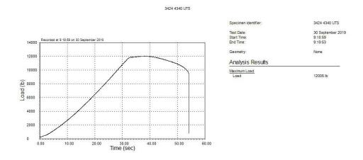
Graph of the ultimate load from the nonheat treated nut. Note the 3/8" grade 8 bolt fractured with no loss of operational properties of the prototype nut.
