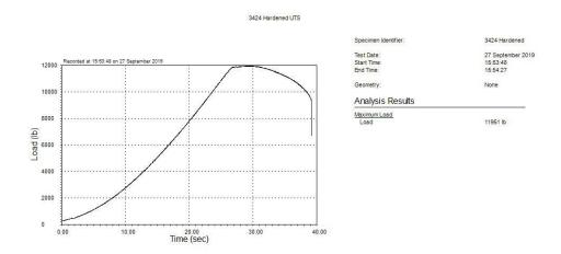
Graph of the ultimate load from the heat treated nut. Note the 3/8" grade 8 bolt fractured with no loss of operational properties of the prototype nut.
