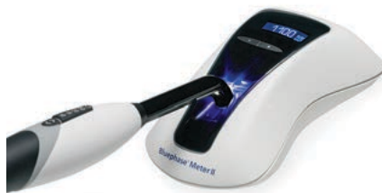
Figure 3: Bluephase Meter II testing a curing light. Photo courtesy of Ivoclar Vivadent.
