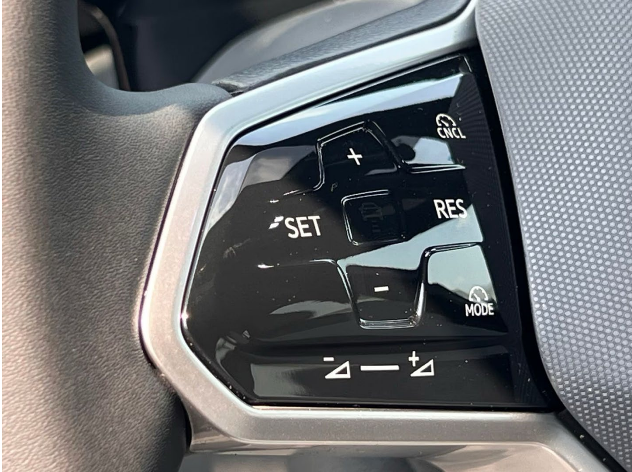
Closeup image of ID.4 Driver Assistance touch controls on steering wheel
