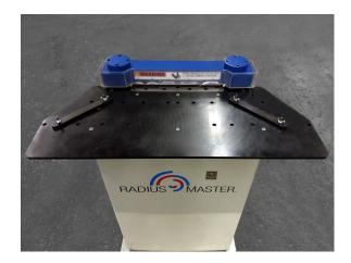
Roper Whitney's Radius Master is a must for every fabricating shop. It's a hydraulically operated, selfcontained unit for making radii in mild steel from 29 gauge up to 7 gauge without having to make blade adjustments and no setup.
