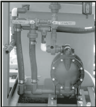
A heavy duty low maintenance air operated pump.
