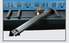
PROTRACTOR for angle shearing.
