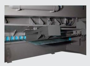
Optional 'heavy duty' hydraulic swing-up (= HDSUB) back gauge stroke 50".
