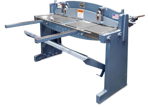
**PEXTO** foot squaring shears are the industry's most accurate. They are easy to operate and offer precise shearing, long life and dependability. Shatterproof transparent finger guards are among their safety features. All are provided with precise gauging and hold-downs for cutting accuracy.
