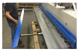
10M14 shears come standard with a full length front sheet support bar for even handling of varying material thicknesses.
