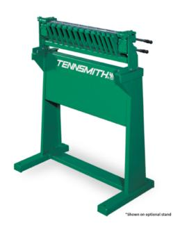
Tennsmith's cleat benders are manually operated tools that form uniform drive cleat edges on rectangular ductwork in seconds without set-up or adjustment. The upper handle forms the cleat and the lower handle opens the tool for easy removal of the material. Heavy cast iron and fabricated steel construction provides long life and trouble-free operation. A TENNSMITH cleat bender can save you time and money.
