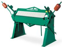
The Model HBU48-12 can handle 12-gauge and lighter materials. The Model HBU72-16 is rated for 6 feet of 16-gauge material. Each hand brake is ideal for both box and pan and straight bending in hot and cold rolled plate, stainless steel, aluminum and heavy plastic.
