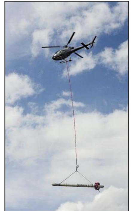
The survey helicopter flew along river paths in the MAP and Chicot regions with an attached electromagnetic instrument housed in a cylinder called a "bird" which was towed about 100 feet beneath the aircraft.
