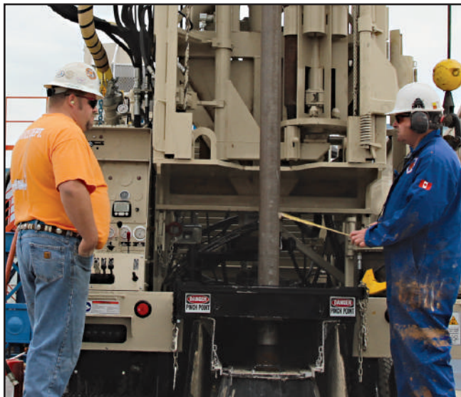
The two most common types of hearing protection used in the drilling industry are foam earplugs and earmuffs. To achieve maximum benefit from either of these hearing protection devices, they must be worn properly.
