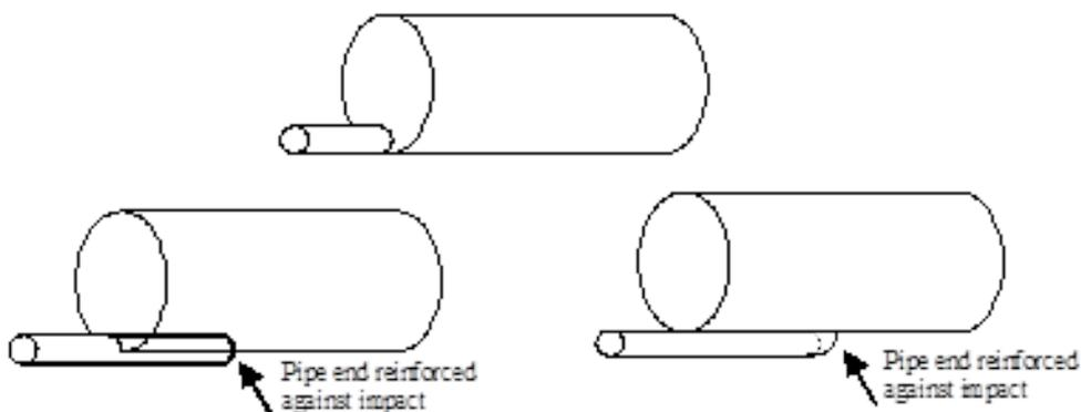
**Acceptable options for pipe connection to holding tank**
