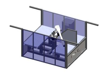
Safety Light Curtains on all 3 Zones 1/4" Table Tops 6x6x3/8 Tube Frame Base 1- Access Door 1- Tip Clean Port
