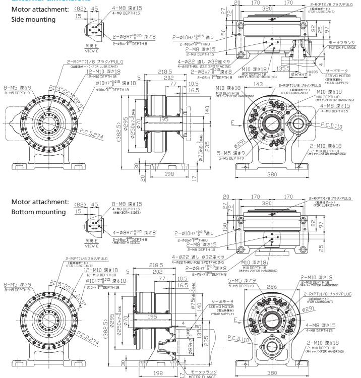
**Precision Reduction Gear RV**<sup>™</sup> **Gearhead equipped with Base Flange** RH-155C Foot Type
