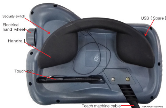
The back and distribution picture of teaching-programming pendant
