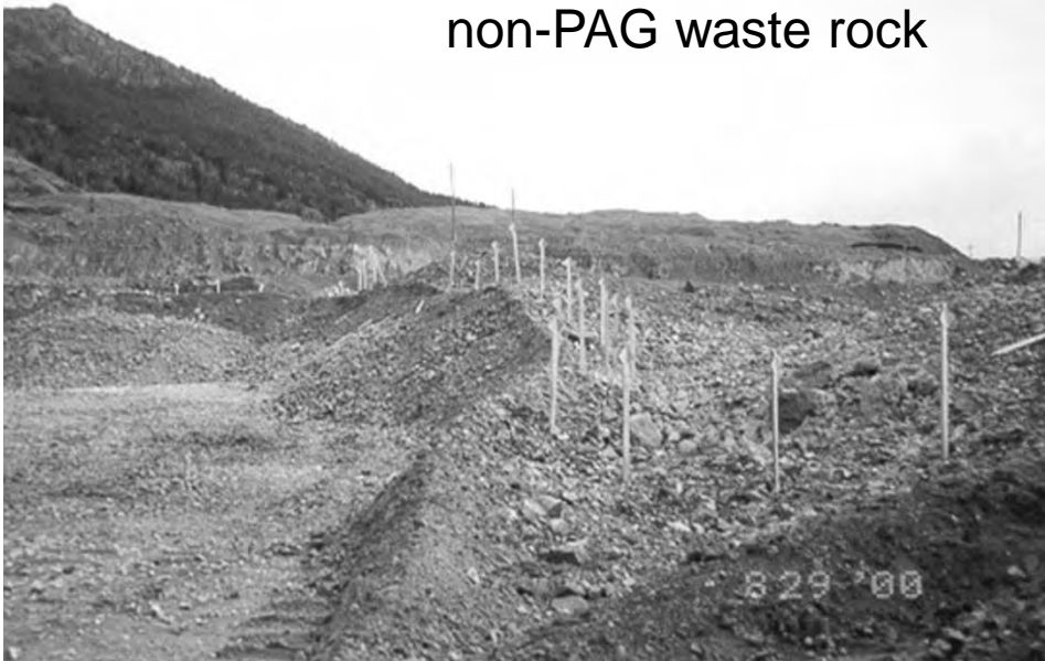
XRF used to ID and segregate low from high-arsenic waste rock
