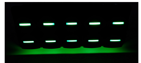
Light "leaking" around the switches. Another major goal was to eliminate the glow around the switches themselves. If the switches were different colors this would cause an undesired mixing effect. I wanted light to only project from the lense that it was intended to.
