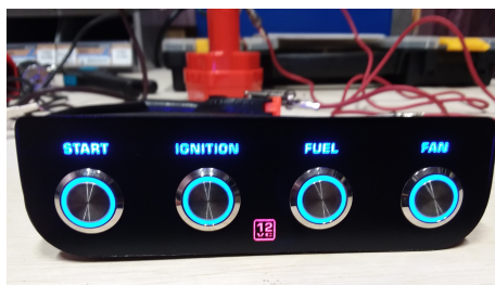
The third variation of a prototype switch panel. Much time was spent to get the lighting to produce minimal glare, and this was not it. There were a half dozen variations after this.
