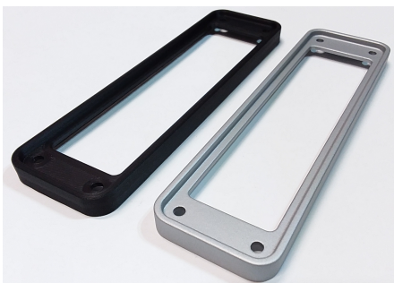
As printed part vs. painted part. Remember to clean paint out of the mounting holes. Too much paint build-up can make too tight a fit.
