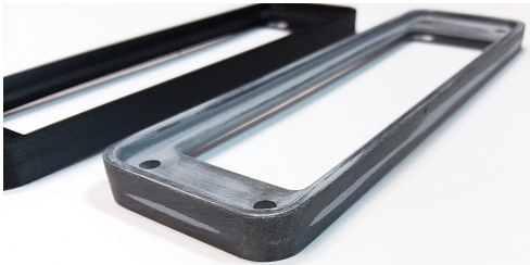
This picture shows a bezel that was sanded with 180 grit, sprayed with primer, then sanded with 320 grit. Notice the gray areas on the sides. These are low spots. More time should have been spent flattening the part before paint. This will show up in the final finish.
