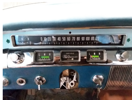
Completed cluster installed in the dashboard of a 1956 Buick Special.
