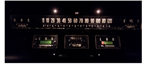
An original 1956 Buick cluster. Notice the stress cracks and foggy areas throughout.
