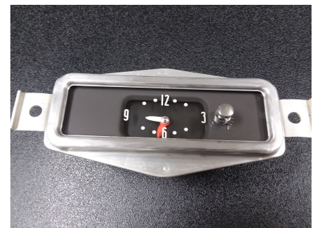
The clock, which was seized up for decades, was also restored and got a new face using the same process.
