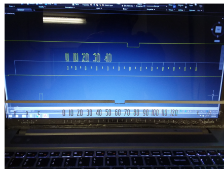
Creating the CAD design with measurements from the original worn out gauge face.
