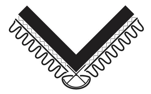
**<u>2.4 End Stop</u>** can be produced to match the rib size and material choice. These can also be mitred to create framing around doors and other penetrations.
