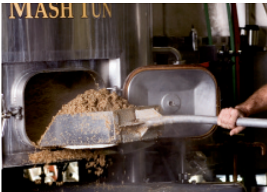
Removing mash—crushed malt steeped in hot water—from the mash tun. Right: Ed Falkenstein (left) and Louis Bruce in the Palmetto taproom
