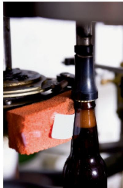
Bottles receive new labels, the final step before beer goes to distribution.
