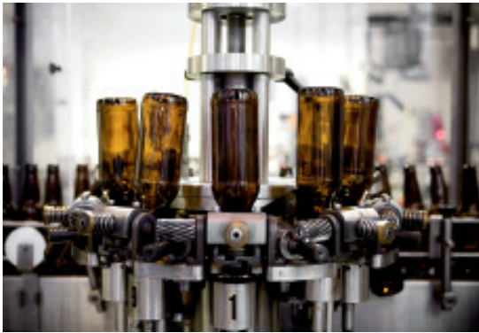
Old bottles undergo a rigorous sterilization process before being refilled.
