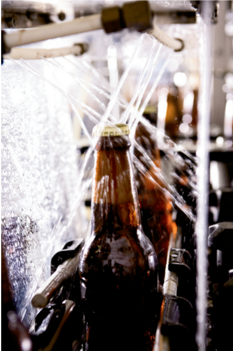
Freshly sterilized bottles are filled with beer, capped, and washed with multidirectional jets of water. The bottles then proceed to a station where they will be labeled before being sent to the distributor.
