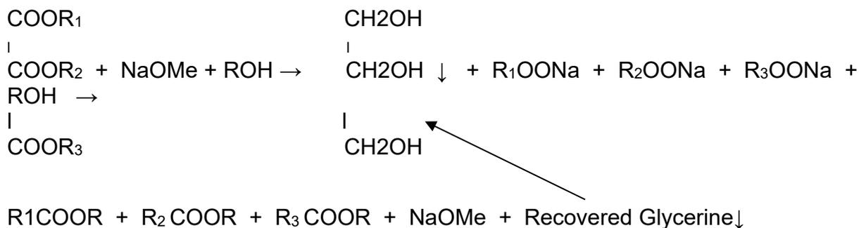
The methyl esters can now be recovered, purified and separated from one another to yield pure cuts of FAME (fatty acid methyl ester). These, in turn can be converted into other, value-added products.
