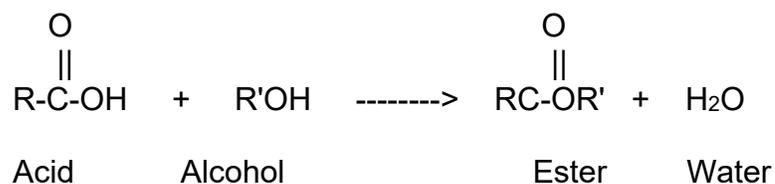
It is necessary to continuously remove by-product water from any esterification process in order to move the reaction toward the formation of the ester.
