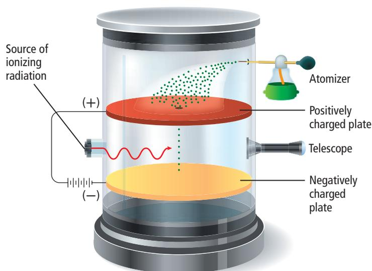
**Figure 4.8** The motion of the oil droplets within Millikan's apparatus depends on the charge of droplets and on the electric field. Millikan observed the droplets with the telescope. He could make the droplets fall more slowly, rise, or pause as he varied the strength of the electric field. From his observations, he calculated the charge on each droplet.
