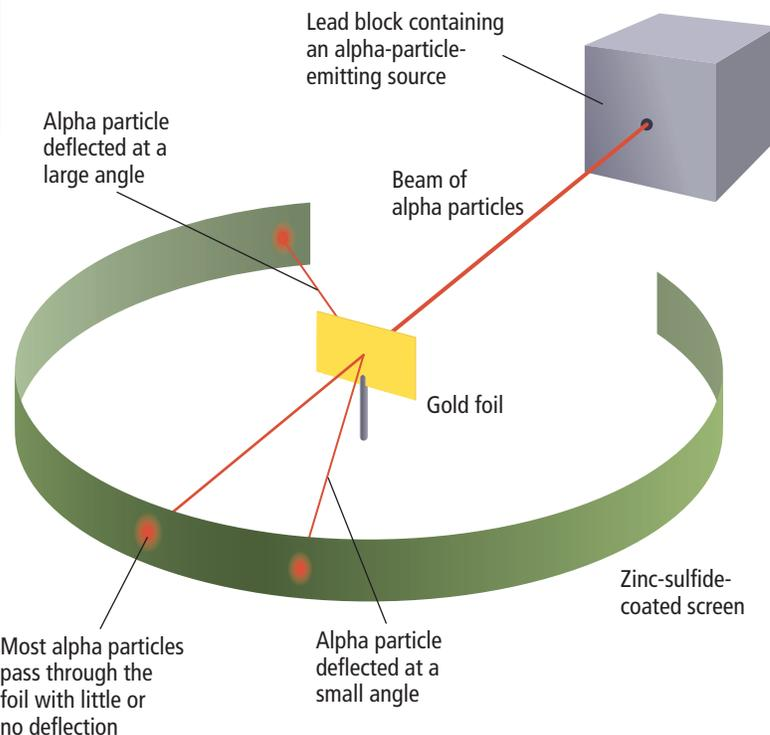
■ **Figure 4.12** During Rutherford's experiment, a beam of alpha particles bombarded a thin gold foil. Most of the alpha particles went through the gold foil. However, a few of them bounced back, some at large angles.
