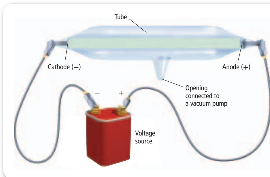
■ **Figure 4.6** A cathode-ray tube is a tube with an anode at one end and a cathode at the other end. When a voltage is applied, electricity travels from the cathode to the anode.
