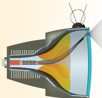
**Television** Television was invented in the 1920's. Conventional television images are formed as cathode rays strike light-producing chemicals that coat the back of the screen.
