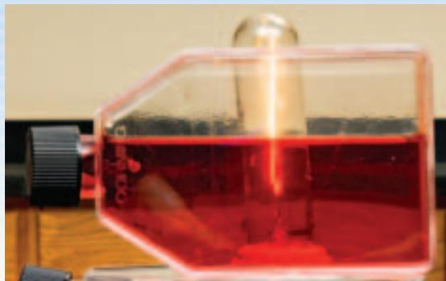
7. With the room lights darkened, view the light using the Flinn C-Spectra®. The top spectrum viewed will be a continuous spectrum from the white lightbulb. The bottom spectrum will be the absorption spectrum of the red solution. Use colored pencils to make a drawing of the absorption spectra you observe.
