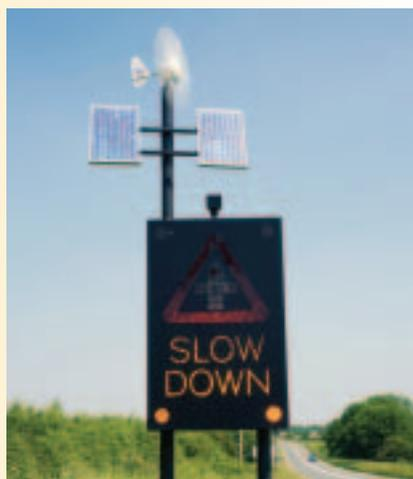
**Solar energy** is sometimes used to power road signs. Photovoltaic cells use the photoelectric effect to convert the energy of light into electric energy.
