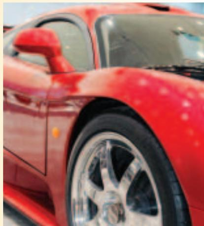
**Chromium** What gives these rims their mirrorlike finish? The metal alloy rim has been plated, or coated, with a thin layer of chromium. Chrome plating has been used in the automobile industry for decades because of its beauty and its corrosion resistance.
