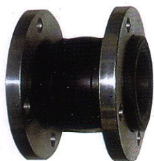
RUBBER JOINT SINGLE SIZE: 1-1/2" ~ 12" STANDARD: ANSI DIN BS MATERIAL: CARBON STEEL PRESSURE: PN6 ~ PN40 150LB ~ 300LB
