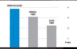
Comparative table of the "R" thermal resistance per inch of thickness of the most common blown insulation
