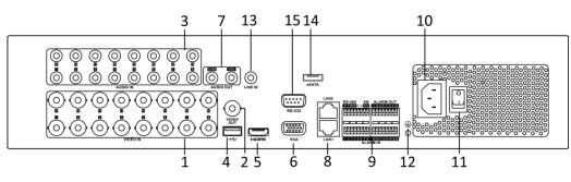
Figure 1.8 Rear Panel of 1080P 2U Chassis Series
