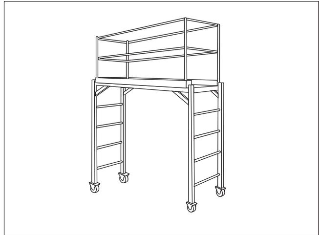
Fig. 3: Manually Propelled Scaffold
