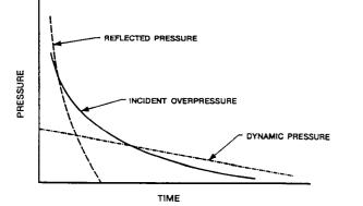
FIG. 2. Blast Wave Characteristics Related to Structural Loadings
