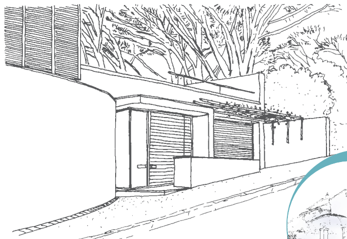
OUT OF SCALE METAL CARPORT AND REMOVAL OF FRONT GARDEN FOR OFF-STREET PARKING BREAKS DOWN STREET EDGE
