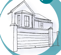
INAPPROPRIATE METAL FOLDING DOOR SET INTO BOUNDARY WALL WHICH DISREGARDS HISTORIC BOUNDARY WALLS, LACK OF SCALE, ETC.
