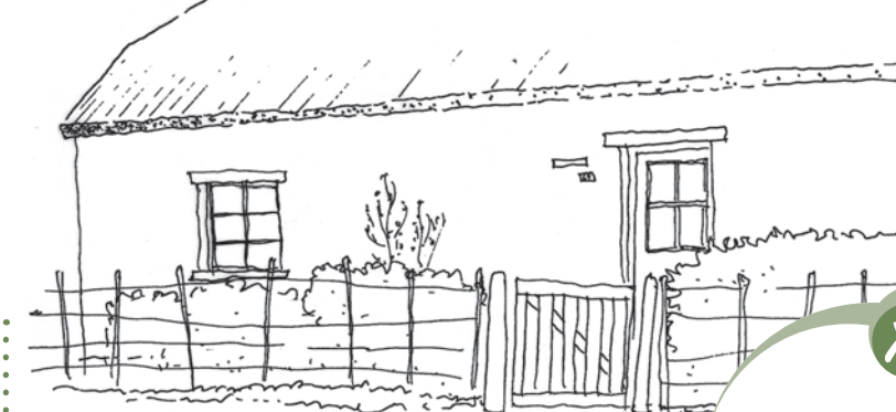
DETAIL OF HISTORIC THATCH-ROOFED MAMRE HOUSE WITH THICK WALLS, SMALL WINDOWS AND DOORS. ROOFS WERE HIPPED WITH CLIPPED ENDS & THATCHED, NOW OFTEN REPLACED WITH CORRUGATED IRON
