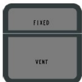
F300SV MINIMUM 12 3/8 X 30 1/8 MAXIMUM 36 X 48 17" VENT HEIGHT
