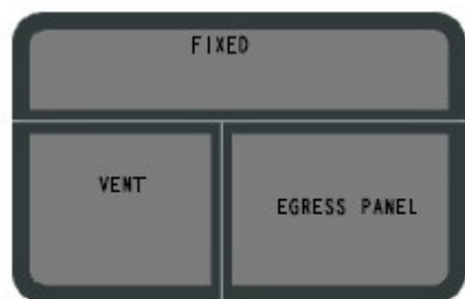
F300SVSE (F300SESV OPPOSITE) MINIMUM 36 1/8 X 30 1/8 MAXIMUM 72 X 48 AT 51 7/8 WIDE & OVER IT BECOMES EQUAL SIDED
