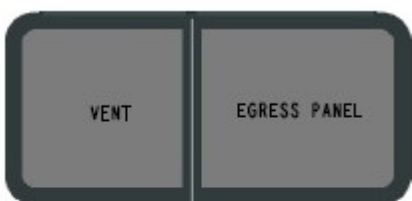
F300FVSE (F300SEFV OPPOSITE) MINIMUM 36 1/8 X 20 MAXIMUM 72 X 30 AT 51 7/8 WIDE & OVER IT BECOMES EQUAL SIDED
