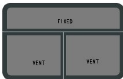
F300SVD MINIMUM 36 1/8 X 30 1/8 MAXIMUM 72 X 48 17" VENT HEIGHT
