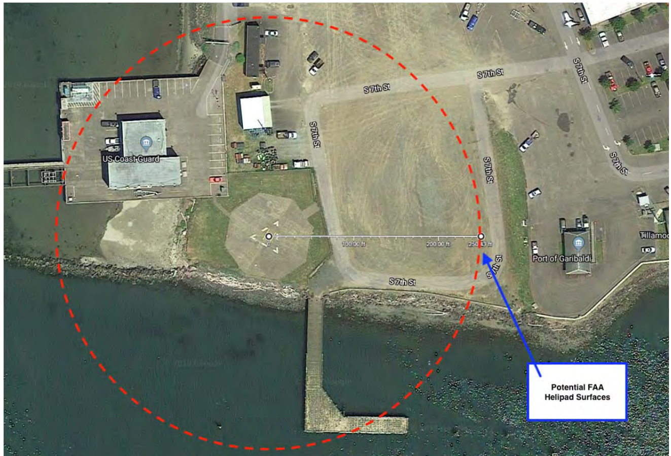
Figure 14: Potential Helipad Approach/Departure and Transition Surface (est. 250 feet)
