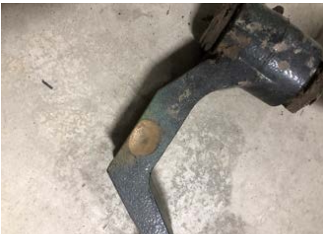
ABOVE: Worn gauge wheel arm (left) and a worn depth equalizer that makes contact to the gauge wheel arm (right).
